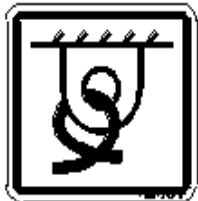
Fig. 6: Label for points used for strapping down the machine
