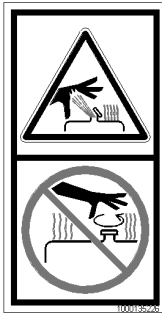
Fig. 18: Hydraulic oil tank under pressure
